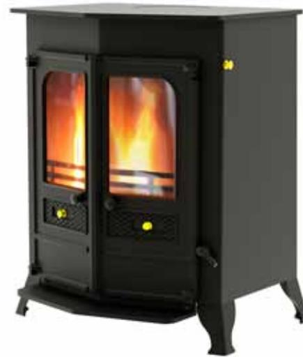
THE COUNTRY 16b Multi-fuel delivers heat suitable for heating domestic hot water plus around 10 radiators. It has a total output of 19.2kW providing 13.7kW to the water and 5.5kW to the room. Once again it is thermostatically controlled with a multi-fuel riddling grate allowing a wide range of solid fuels to be burnt. Its deep fire bed allows solid fuel to be loaded up for excellent overnight burning performance.
