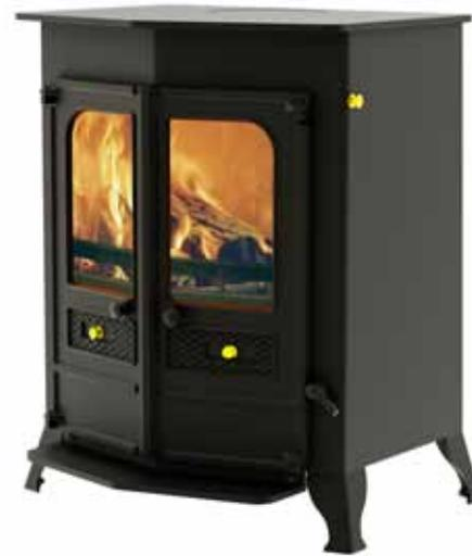
THE COUNTRY 16b Woodburner is a fully fledged biomass central heating boiler. The total output is 15.4kW; 8.2kW to the water and 7.2kW to the room. This model will run around 7 radiators and supply all domestic hot water. It features the riddling grate to ensure easy ash removal and Charnwood's standard clean burn technology for ultra efficient burning.
