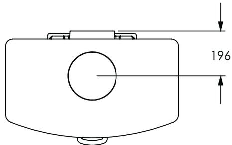
Flue Outlet To Suit 175mm (7") Flue Pipe
